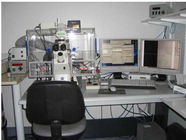
*Microscopie confocale, LSM510META (Carl Zeiss)*
